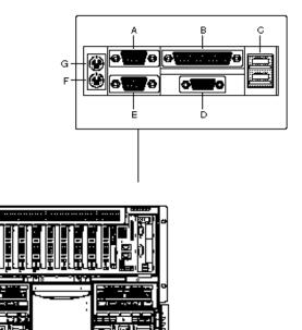
Figure 3-6: Riser Board External I/O Connectors
